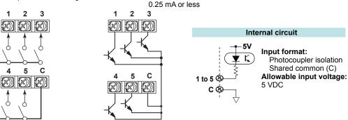
Withstand voltage: 500 VDC for one minute (between input terminals and the ground terminal)
